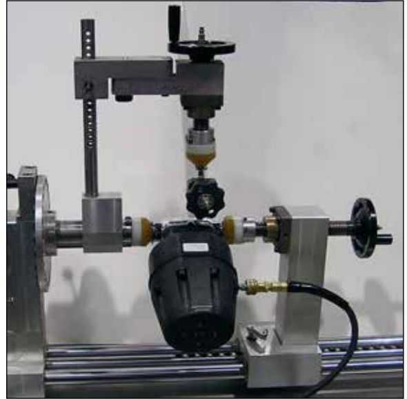
Leak and Shell Test
